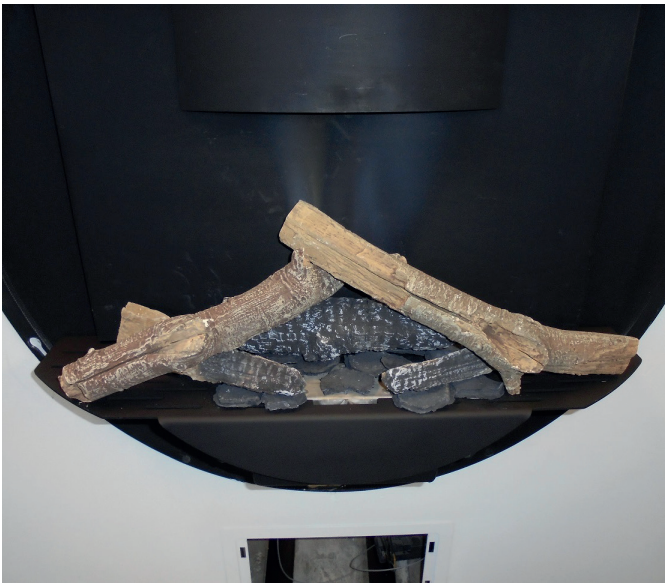
Position Logs G1 & S2 as shown in the diagram. Scatter the Glow Strands among the Logs and Embers. Finally Check the appliance for Pilot ignition and cross lighting ensuring that no material is impinging the operation of the Pilot.
